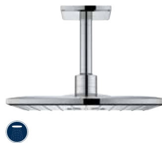
26 481 000 / 26 484 000 Head shower set Rainshower 310 SmartActive length 142 mm 2 spray patterns: GROHE PureRain, ActiveRain WELS 3 stars, 9 ltrs/min
