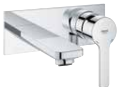
19 409 001 / 23 571 000 M-Size Basin mixer wall mounted, 149mm + separate concealed body WELS 3 stars, 9 ltrs/min
