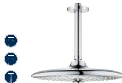
26 460 000 Euphoria 260 Ceiling shower arm projection 142mm 3 spray patterns: Rain, SmartRain, Jet WELS 0 star, 9.5 ltrs/min
