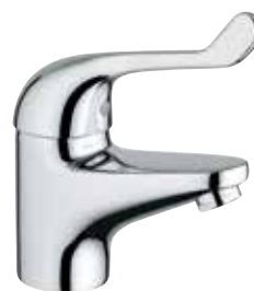
32 789 000 Euroeco Special Single-lever safety basin mixer ½ Single hole installation Adjustable flow rate limiter Laminar flow straightener 9 ltrs/min Metal lever 120mm Temperature limiter WELS 0 star, 9 ltrs/min
