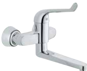
32 793 000 Euroeco Special Single-lever safety basin mixer, ½" wall-mounted adjustable flow rate limiter cast swivel spout, lockable laminar flow straightener 9 ltrs/min projection 256mm metal lever 170mm temperature limiter WELS 0 star, 9.5 ltrs/min
