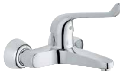
32 795 000 Euroeco Special Single-lever safety basin mixer, ½" wall-mounted adjustable flow rate limiter cast spout laminar flow straightener 9 ltrs/min projection 204mm metal lever 170mm temperature limiter WELS 0 star, 9.5 ltrs/min
